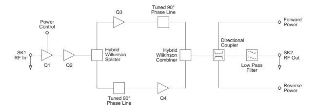
Figure 2.2 T828 RF Circuitry Block Diagram
