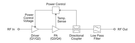
Figure 2.1 T828 High Level Block Diagram
