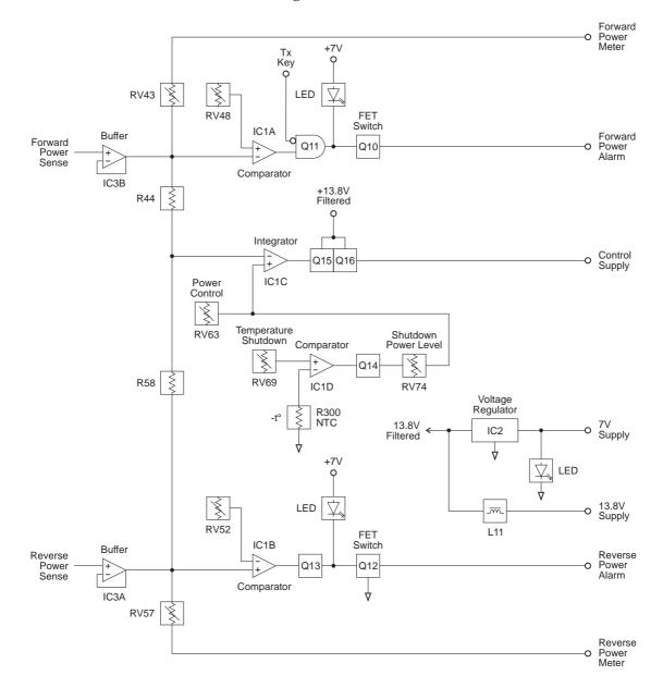
Figure 2.3 T828 Control Circuitry Block Diagram
